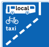
With-flow bus lane ahead which pedal cycles and taxis may also use
